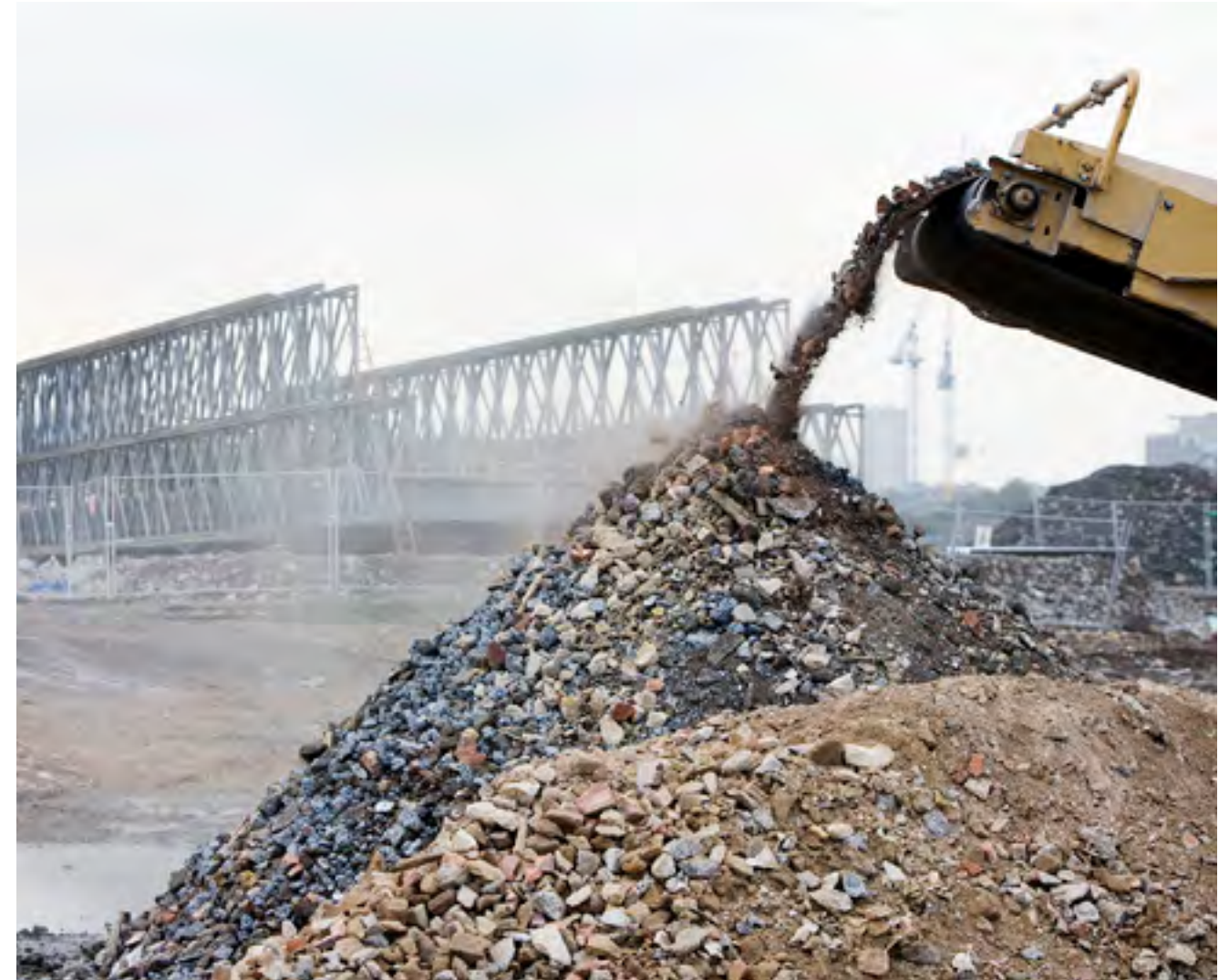
Conveyor belt on plant designed to reuse concrete from demolished buildings on the London 2012 Aquatics Centre site.
